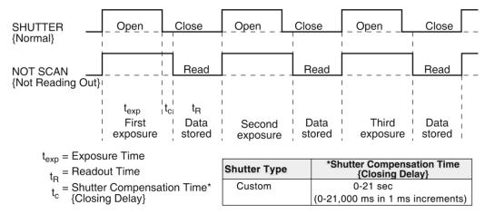
Figure 29. Free Run {No Response} Timing Diagram
